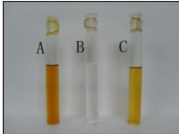
Comparison between the concentrate (A), permeate (B) and feed solution (C) at the end of the experiment
