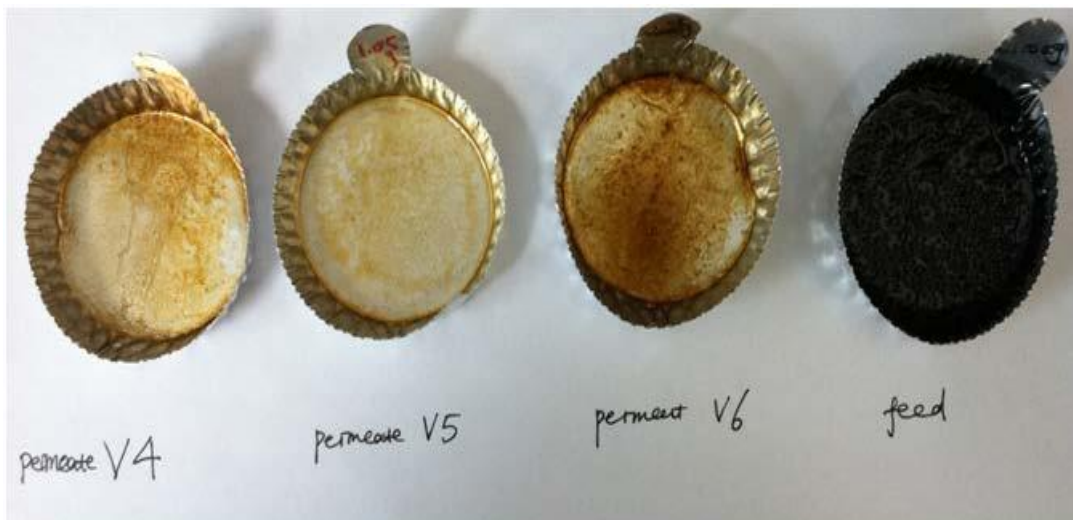
Permeate samples from the V4, V5, V6 membranes, and feed
